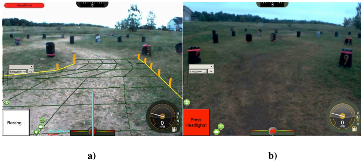
Figure 4.5. Operator control unit interface with (a) and without (b) driver feedback
