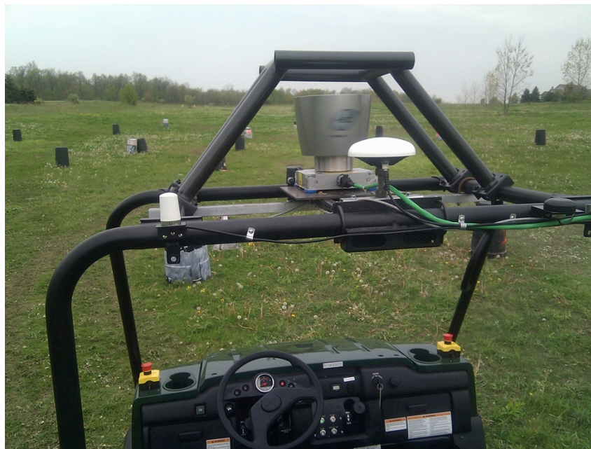
Figure 4.3. LIDAR, GPS, and communication antennae
