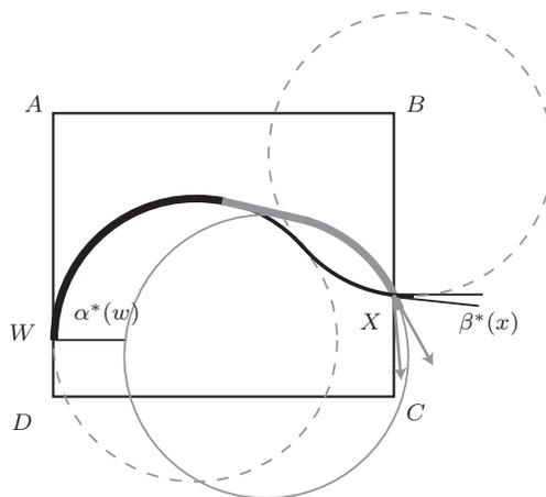
(c)  $\overline{\beta}(x) < \beta^*(x)$ , originally defined  $\Pi_x$  (the path in black) is not admissible,  $\Pi_x$  redefined as a  $C^+SC^+$  path (shown in gray).
