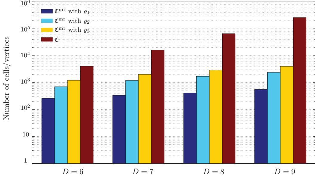
**Figure 7.11:** Comparison of the number of vertices in the topological graphs associated with multi-resolution cell decompositions with different window functions and with the finest-level cell decomposition  $\mathcal{C}$ .
