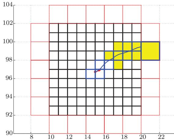
(a) Intermediate iteration: local perspective. The vehicle's configuration at this iteration is indicated by the red-colored marker and arrow. The  $x$  and  $y$  axes indicate inertial position coordinates, in kilometers.
