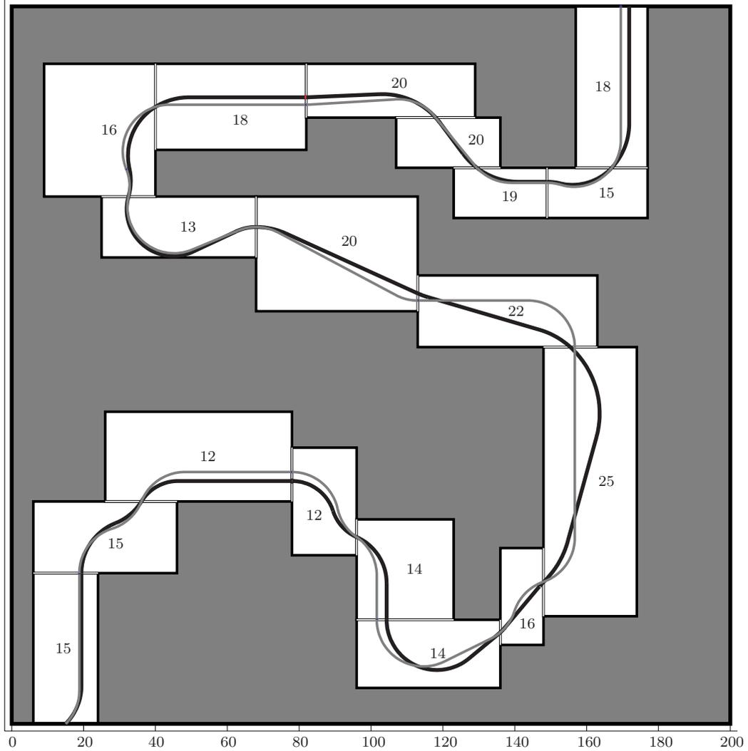
**Figure 7.15:** Path planning through a channel: The gray path has a constant curvature bound of 13 units, while the black path has variable curvature bound. The numbers within each rectangle indicate local curvature bounds for the latter.
