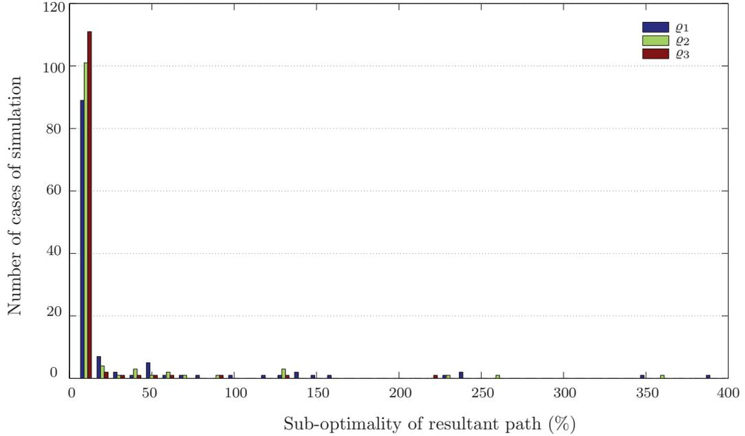
**Figure 7.10:** Histogram showing the distribution according to percentage sub-optimality of simulated cases, for different window functions. Whereas the sub-optimality was restricted to less than 20% for most cases for all window sizes, note that the “largest” window function  $\varrho_3$  has the fewest cases of highly sub-optimal results.
