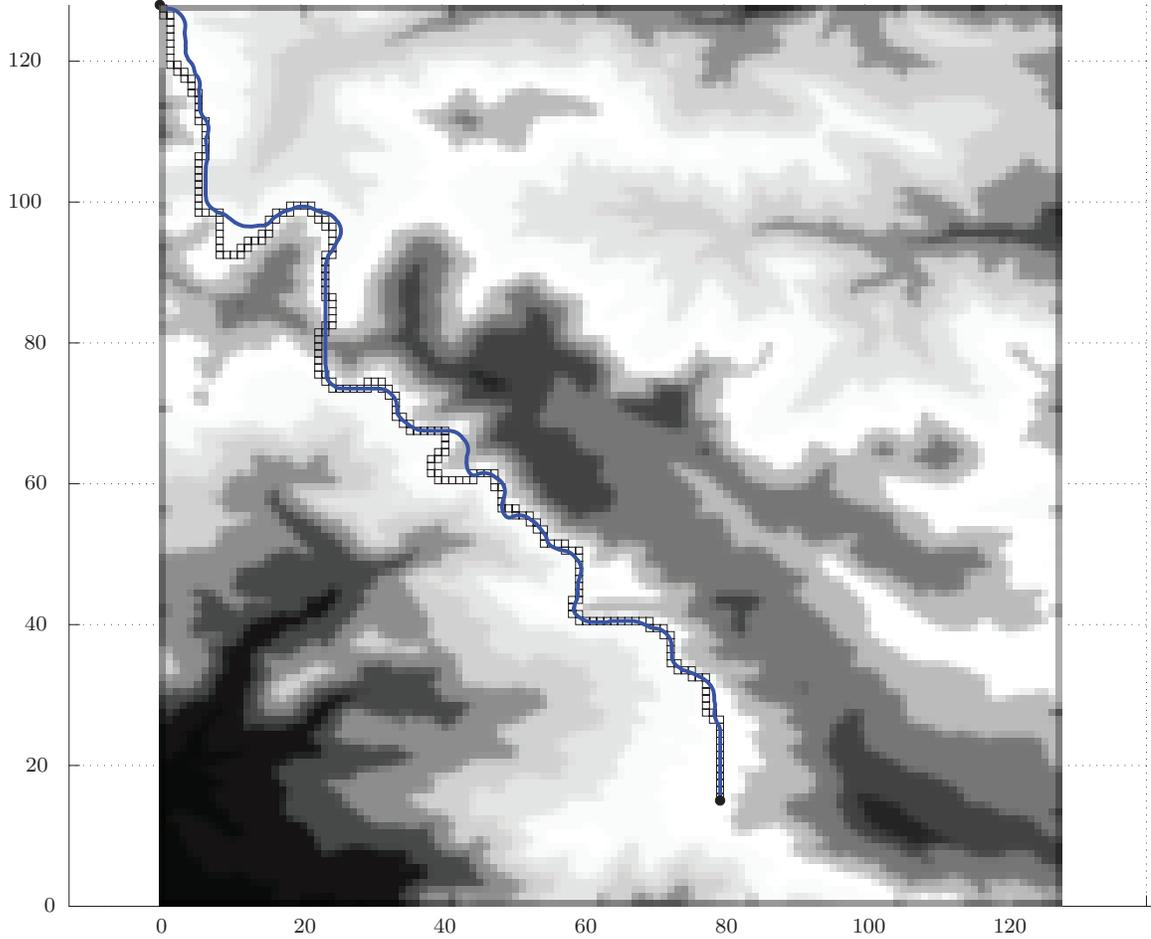
**Figure 7.12:** Result of motion planning simulation using the aircraft navigational model. The blue curve is the geometric path corresponding to the resultant state trajectory, while the channel of cells in black is the result of executing A\* algorithm (without incorporating vehicle dynamical constraints). The initial position is at the top left corner of the map. The units for the  $x$  and  $y$  axes are kilometers.
