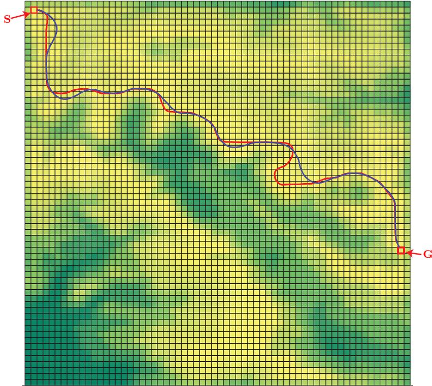
**Figure 7.7:** Application of proposed motion planning framework for finding “low-elevation” paths: lighter areas represent more favorable regions of the workspace. The Dubins car kinematical model is used in TILEPLAN. The red curve represents a path with  $r = 1$ , whereas the blue curve represents a path with  $r = 2$ .
