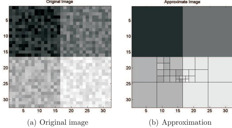
**Figure 6.5:** Example of multi-resolution decomposition using the approximation (6.7).
